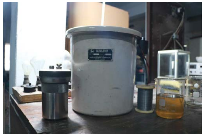
Fig.3 Bomb calorimeter used for the experimentations.
